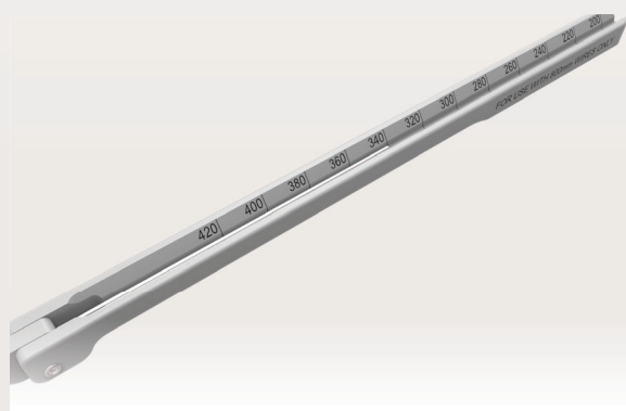
FIGURE 18: Read the measurement from the back of the wire.
